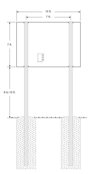
Once you have verified the positions of the posts and the size of the footings, you are ready to dig your holes, pour your concrete, and set your posts. There are several techniques for ensuring proper alignment of the posts. Typically installers will construct a temporary wooden support frame to hold each post in place while the concrete sets. Having plumb posts in the proper position is the key to a smooth mechanical installation.
